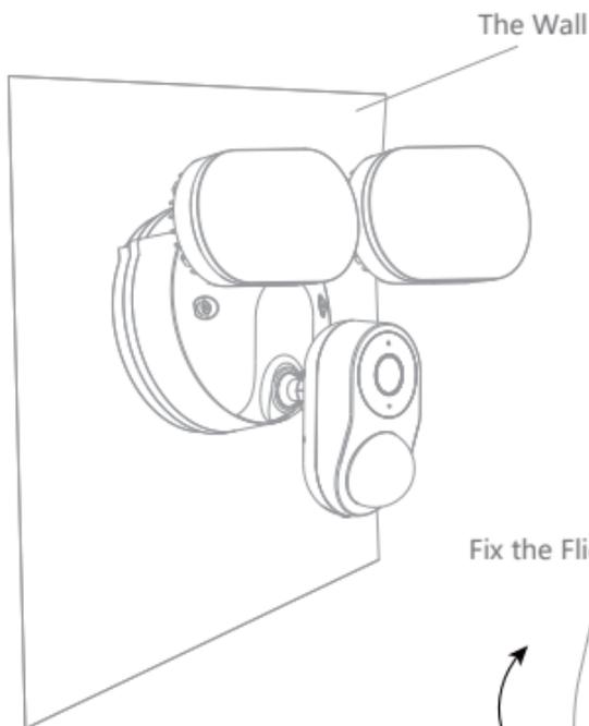
Fix the Flight Cam to the bracket
