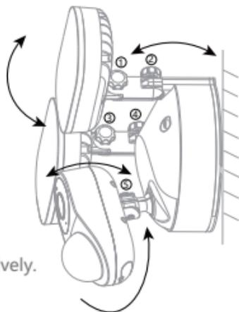
1. After fixing camera on the wall, adjust the camera angle according to the arrow directions.
