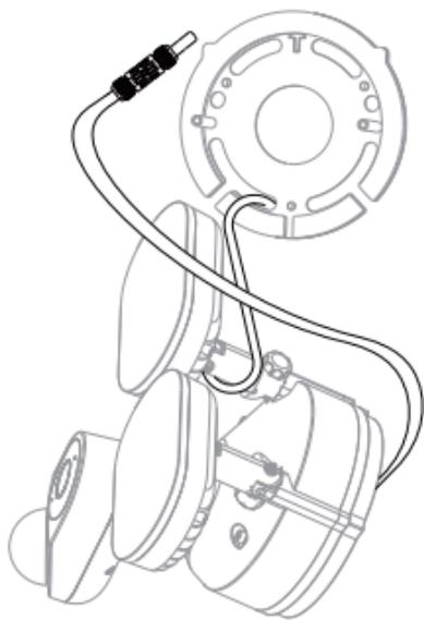
Hook one end of the provided hook into one of the mounting holes on your Bracket.
